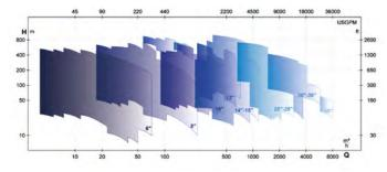
Radial & semi-axial impeller working ranges (60 Hz)
